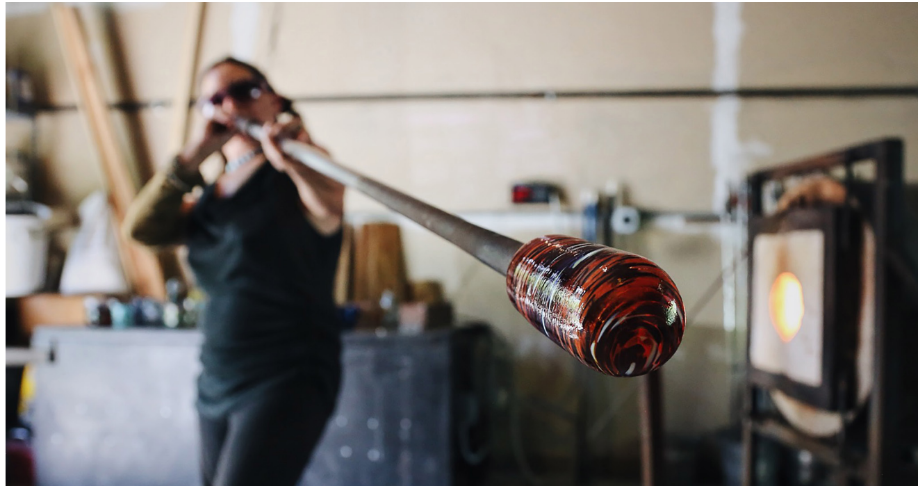
Muñoz begins by blowing air into the molton glass.. Photo credit - Samantha Yancey
